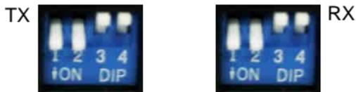
Setting the Transmitter and Receiver group ID via the 4-bit DIP switch. The correspondent receivers are required to switch to the same ID as the receiver. It can set up maximum 16 Group IDs. Reboot the system to apply the group setting.
