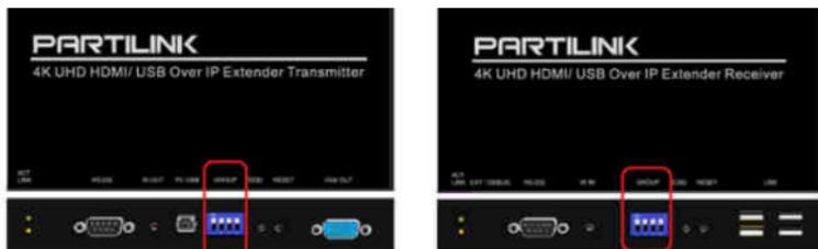
Figure 46. Transmitter and Receiver Unit Grouping
