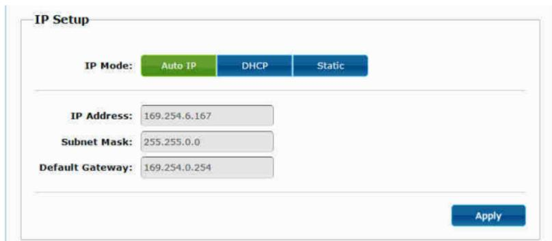
The screenshot shows the 'IP Setup' configuration page. At the top, there are three buttons for 'IP Mode': 'Auto IP' (highlighted in green), 'DHCP' (blue), and 'Static' (blue). Below this, there are three input fields: 'IP Address' with the value '169.254.6.167', 'Subnet Mask' with '255.255.0.0', and 'Default Gateway' with '169.254.0.254'. An 'Apply' button is located at the bottom right of the form.
